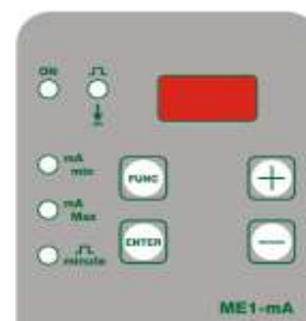
Chlorine dosing pump model ME1-mA receiving the 0-4/20 mA signal from the MS-MP controller
